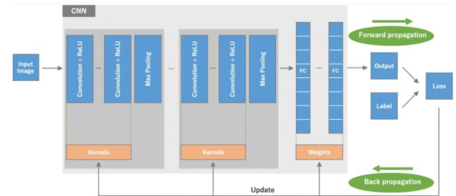
Fig. 1. Convolutional neural network (CNN) architecture and the training process
